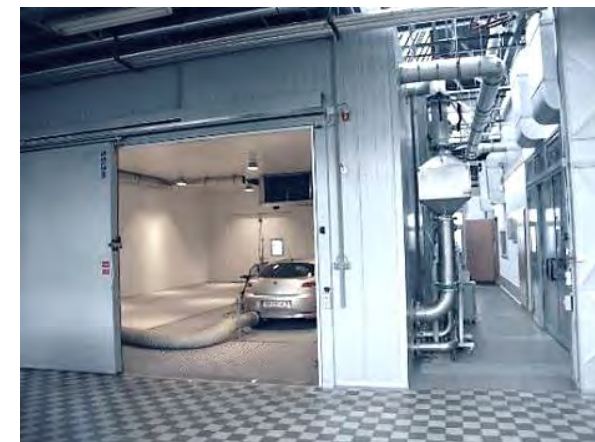
Climatic chamber (-35°C to +60°C) 14,3×10,1×4,3 m
