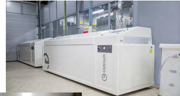
Large-dimension climatic chamber 3x7x9 m
