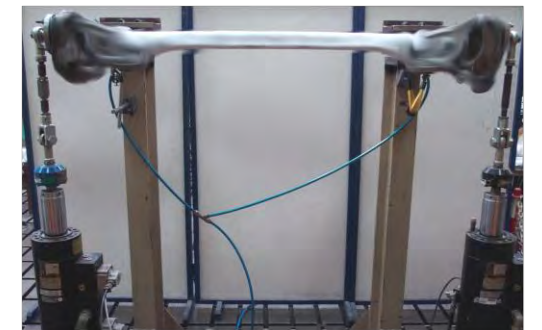
Durability test – multiaxial load
