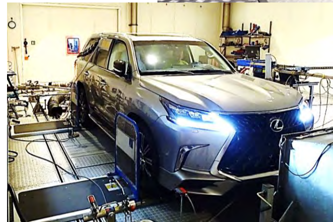
Chassis dyno facilities for vehicles with ICE and hybrid powertrains
