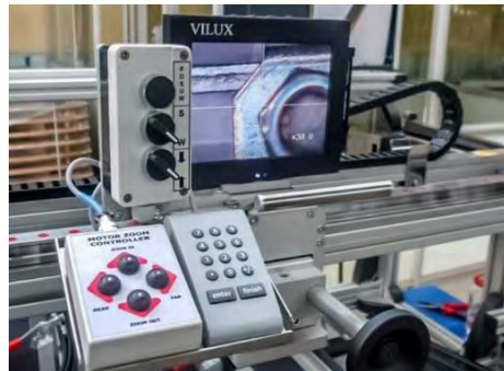
Non contact, optical device for the control of gaskets with automatic recording and data transmission
