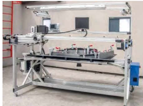
Non contact, optical device for the control of gaskets with automatic recording and data transmission
