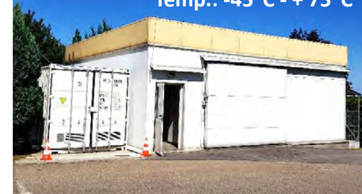
Large dimension climatic chamber Temp.: -45^{\circ}\text{C} - +75^{\circ}\text{C}
